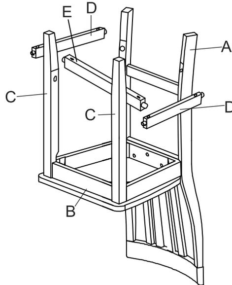
Step 4. Finger-tighten bolts (part #2), do not overtighten. Secure stretchers (parts D & E) using screws (part #7) and phillips head screwdriver.
